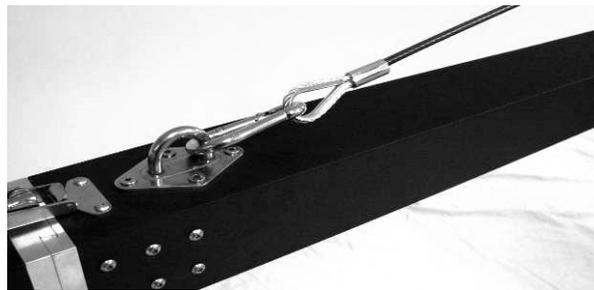
Ext. Cable 2 – clip the end with the turnbuckle to the latch point closest to the front of the crane. Place the cable over the cable guide and secure the simpler end to the latch point it can reach closest to the rear of the crane.
