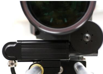
Front view of TOC motors mounted horizontally
