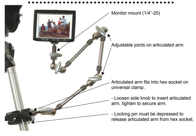
Universal clamp – can be adapted for use with flat surface (e.g., table) or round bar (e.g., tripod) by adding or removing wedge-shaped **saddle** (included). Remove saddle for clamping on round bar.
