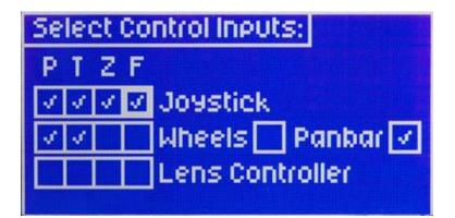
Here is where you can assign how Pan, Tilt, Zoom, and Focus will be controlled. Move the cursor box to where you'd like to control each axis. **Note:** Make sure you have the correct controller selected. I.E. if you are using wheels, make sure "wheels" is selected rather than "panbar". This will greatly effect the performance of the Head.
