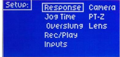
When pressed while already in the setup menu, the "menu" button will enter a second setup menu.
