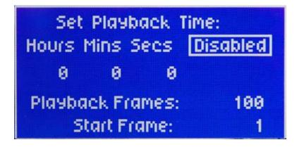
The intervalometer has three modes. "Playback Time Mode", "Playback Ratio Mode", and "Stop Motion Mode".
