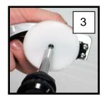
Un-screw (A) the Focus ring gear and then placing it around the focus ring on the camera, then re-attach the screw and tighten until snug (B). Be sure that focus ring gear is lined up centered & symmetrically with the Focus ring on the Camera (C).
