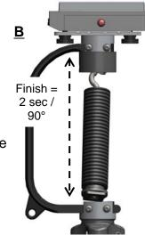
8) <u>Check Vertical Balance</u> - Walk with the unit and move it side to side and front to back. If the unit is vertically balanced, it should stay upright when moved - it should not sway or behave like a pendulum. If the unit sways, adjust the vertical balance until the unit stays vertical while in motion.
