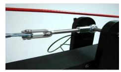
Make sure black cable is on this side of the cable guide to clear the red cables.
