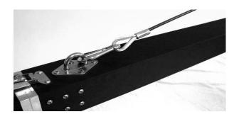
Ext. Cable 2 – clip the end with the turnbuckle to the latch point closest to the front of the crane. Place the cable over the cable guide and secure the simpler end to the latch point it can reach closest to the rear of the crane.
