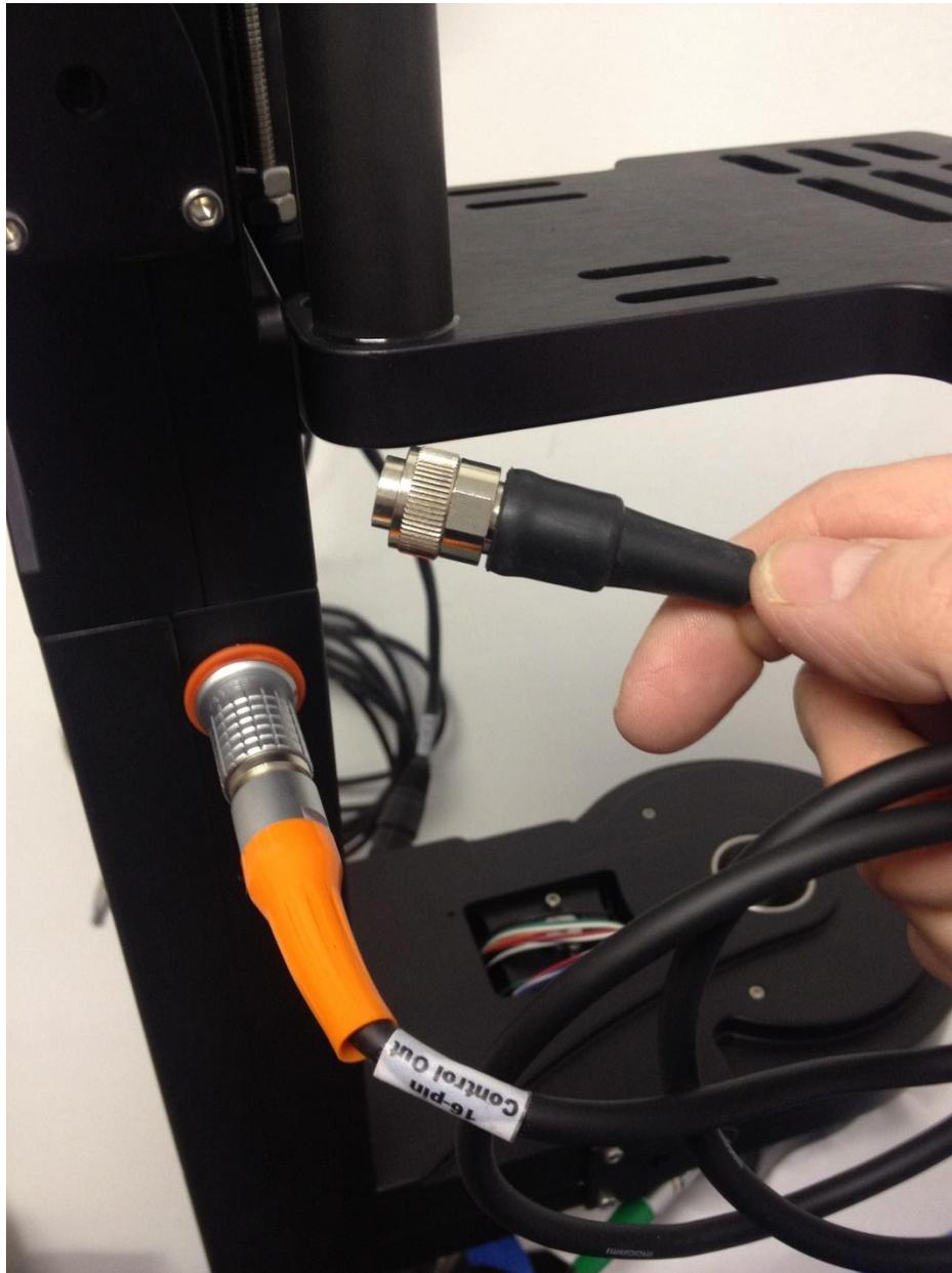
VZCP-C09 (\$399 each) – Lens control cable. **MUST** be optional, because there are **MANY** different types of connectors and software protocols. Head outputs lens control via 16pin 2B Lemo. **Customer must specify connector type and lens model at time of order.**
