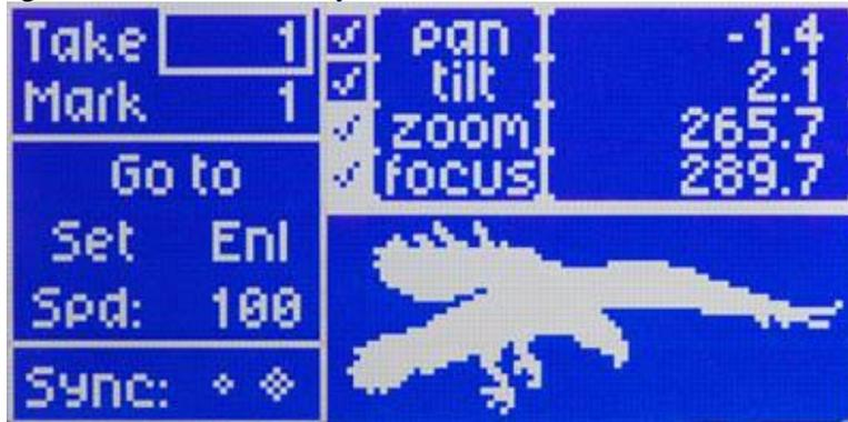
The upper right portion of the LCD screen shows motor status and current positions for pan, tilt, zoom and focus. A check in the box to the left of the axis name indicates that that motor is enabled to run. If soft limits are enabled for the axis, the box is filled and appears white with a blue check mark. The numbers to the right of the axis names are the motor positions; pan and tilt are shown in degrees, and zoom and focus are shown as an unscaled number from 0 to 1000.
