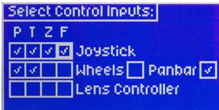
Here is where you can assign how Pan, Tilt, Zoom, and Focus will be controlled. Move the cursor box to where you'd like to control each axis.
