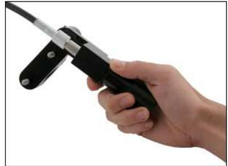
5. Attaching the drive cable to the focus block is essentially the same as described in steps 3 & 4 (*note: focus block may differ from the one pictured*). Align the flat-head tip of the cable with the slot in the threaded socket located on the focus block. Insert the flat-head tip and hold the cable in place, turning the focus control handle until the whole unit moves smoothly – at this point the brass gear on the focus block should easily turn the focus ring on the lens.
