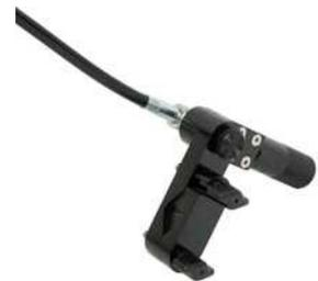
1. Affix the focus control handle to your tripod pan handle using the adjustable clamp. Once the clamp is firmly tightened, you can adjust the orientation of the focus control handle by loosening the screw at the locking swivel joint.
