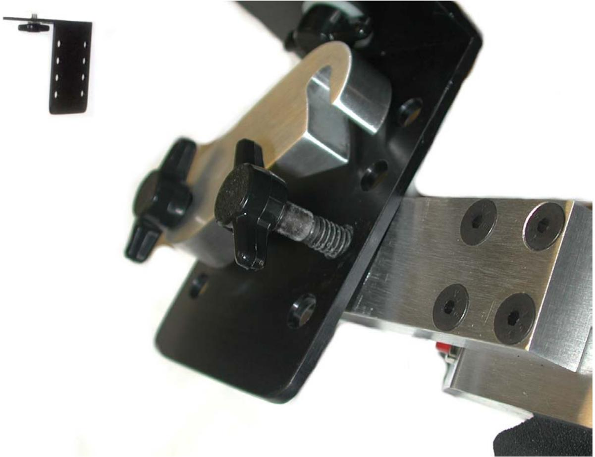
Assembly to controller- Remove the two bolts on the controllers clamp. Take the PGB and 'sandwich' it between the controller and the clamp. Replace the bolts through the PGB bracket holes. You can adjust the height of the bracket by lining up the appropriate holes.
