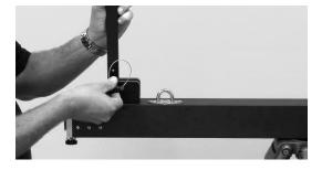
Pull the pin out from the cable guide baseblock. Lift the cable guide and insert the pin to secure.
