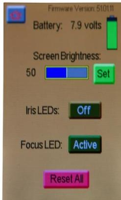
The system menu is where you can monitor battery output, as well as adjust screen brightness, toggle LED's on/off, or reset all parameters if needed. If screen brightness is adjust to 100, it will enter “daylight mode”, which will change the color scheme to be more visible in extreme brightness.
