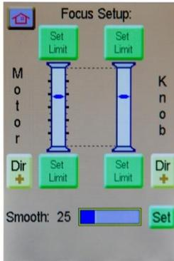
From the Focus Setup screen, you can set the focus motor and focus knob limits, reverse motor and knob response direction, as well as adjust smoothing.
