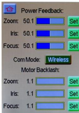
The setup menu is where you can adjust power feedback, Com Mode, and Backlash compensation for each individual motor.
