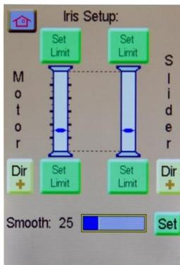
From the Iris Setup screen, you can set the iris motor and slider limits, reverse motor and slider response direction, as well as adjust smoothing.
