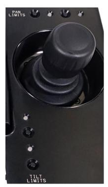
2) You can also set the limits in the <u>Axis Setup</u> menu. In this case, move the head to each end and press "Set Limits" on the touchscreen. Here you can also change the deceleration setting, which softens the 'braking' action when you run into the limits. The same limits setup applies for focus (when available on the lens in use):
