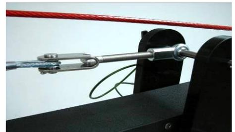
Make sure black cable is on this side of the cable guide to clear the red cables.
