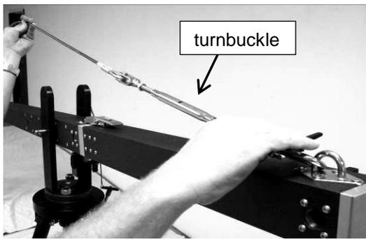
Next, place the cable over the cable guide and secure the other end to the latch point at the front of extension section 1.
