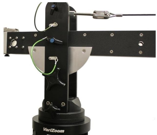
**\*\*\*Option:** If you want to reduce the amount of counterweight needed in SnapCrane-16 mode, you can shift the brake plate forward so you can use the front pivot hole – this will minimize the amount of counterweight needed at the back of the crane.
