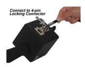
Connect the <u>4-pin</u> XLR power cable from the AC adapter to the <u>4-pin</u> XLR power connector located on the MC50 Control Unit.
