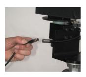
Connect the other end of the <u>4-pin</u> control cable to the MC50 Control Unit at the locking <u>4-pin</u> connector. The additional <u>3-pin</u> port located beneath the motor cable port will provide 24VDC power output.
