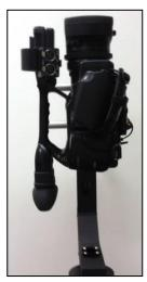
Engage the brass motor gears to the black arm gears and tighten. Be sure the levers are pointing away from the rotating arm.
