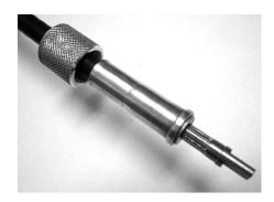
4. At this point, slide the threaded metal cap onto the threaded socket and tighten thoroughly.
