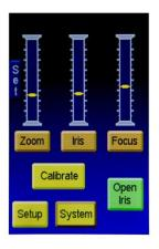
From the Home Screen, you can monitor the current lens positions as well as enter the setup screens for Zoom, Iris, and focus. You can also enter the Control, Calibrate, Setup, and System menu screens. From this screen tap "Open Iris" to fully open iris. Tap the button again to return the iris motor to the location of the iris slider. There is also a "Set" button that will recalibrate the zoom toggle in case it starts to drift.
