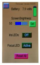
The system menu is where you can monitor battery output, as well as adjust screen brightness, toggle LED's on/off, or reset all parameters if needed. If screen brightness is adjust to 100, it will enter "daylight mode", which will change the color scheme to be more visible in extreme brightness.
