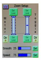
From the Zoom Setup screen, you can set the Zoom motor and zoom Toggle limits, reverse motor and Toggle response direction, as well as adjust Zoom speed and smoothing.
