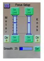
From the Focus Setup screen, you can set the focus motor and focus knob limits, reverse motor and knob response direction, as well as adjust smoothing.
