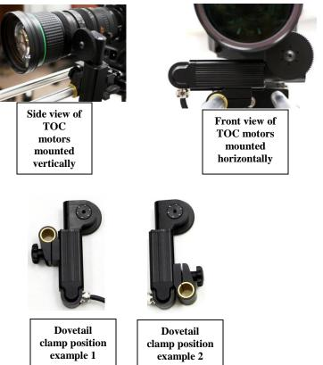
After the motors have been mounted on the rods, secure the gears against the proper lens rings and tighten the dovetail clamps. Mount your TOC receiver and attach the antenna. **First** plug the lens motors into TOC receiver according to their function (yellow to yellow, zoom to zoom, etc)
