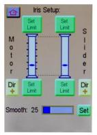
From the Iris Setup screen, you can set the iris motor and slider limits, reverse motor and slider response direction, as well as adjust smoothing.
